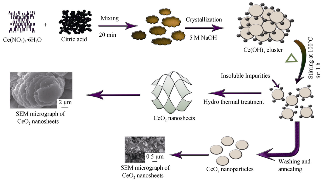
Fig. 4. Illustration of the growth mechanism of \text{CeO}_2 nanostructures.
