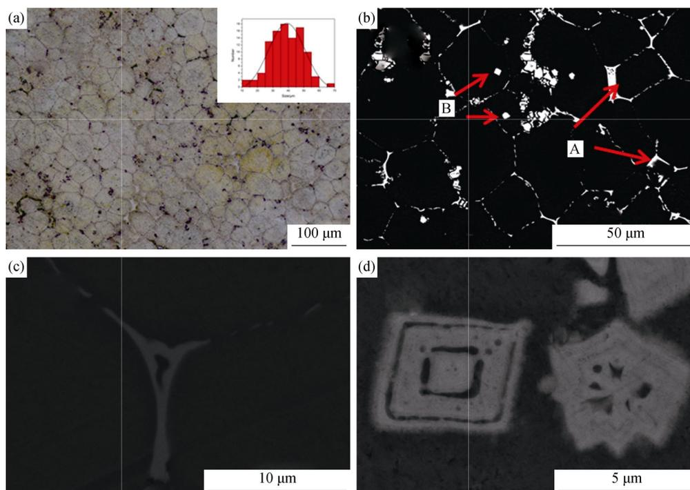
**Fig. 1.** Microstructures of the as-cast ingot: (a) optical microscopy image; (b) back-Scattered electron image; (c) eutectic structures; (d) primary Al<sub>3</sub>(Sc,Zr).
