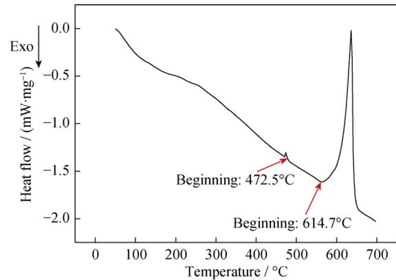
**Fig. 3. DSC curve of the as-cast alloy.**
