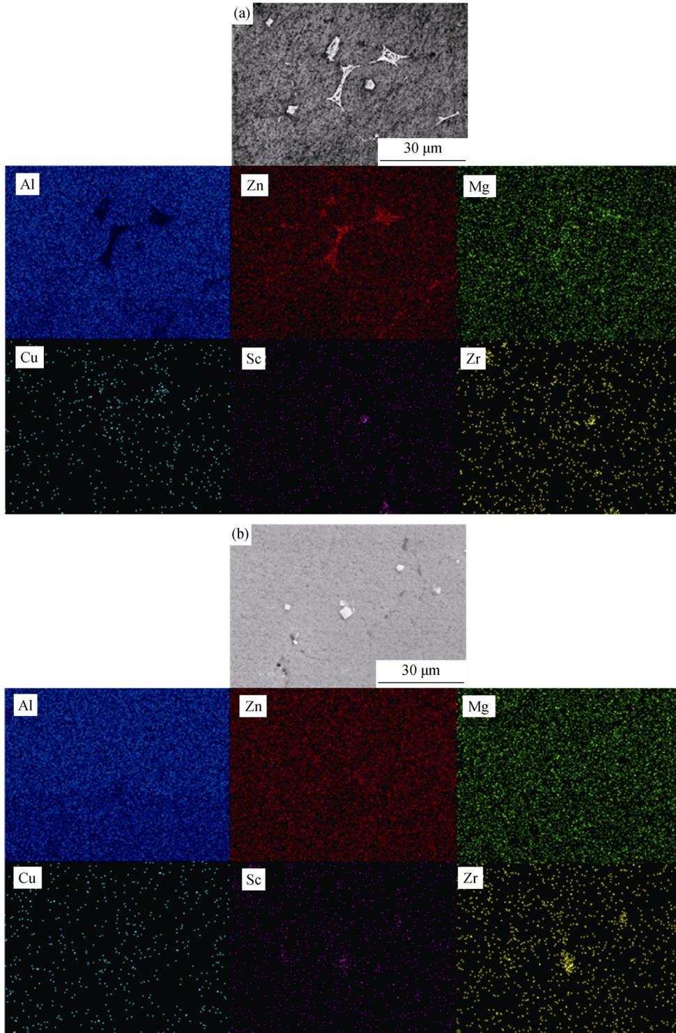
Fig. 6. EDS maps of the as-cast alloy (a) and the alloy homogenized for 1 h (b).
