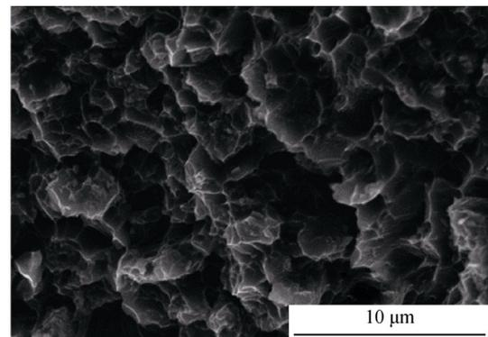
Fig. 8. SEM micrograph of the extruded alloy.
