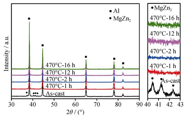
**Fig. 4. XRD patterns of the as-cast specimens at different homogenization conditions.**
