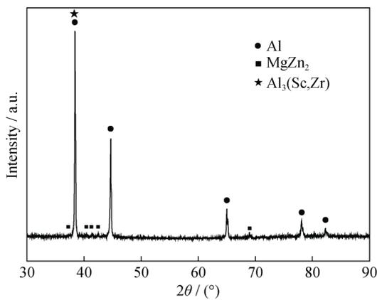
**Fig. 2. XRD pattern of the as-cast alloy.**
