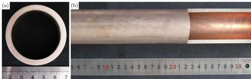
Fig. 11. Surface morphology of BFe10 cast tube with the optimal process parameters: (a) transverse section of the tube and (b) external and internal surfaces of the tube.
