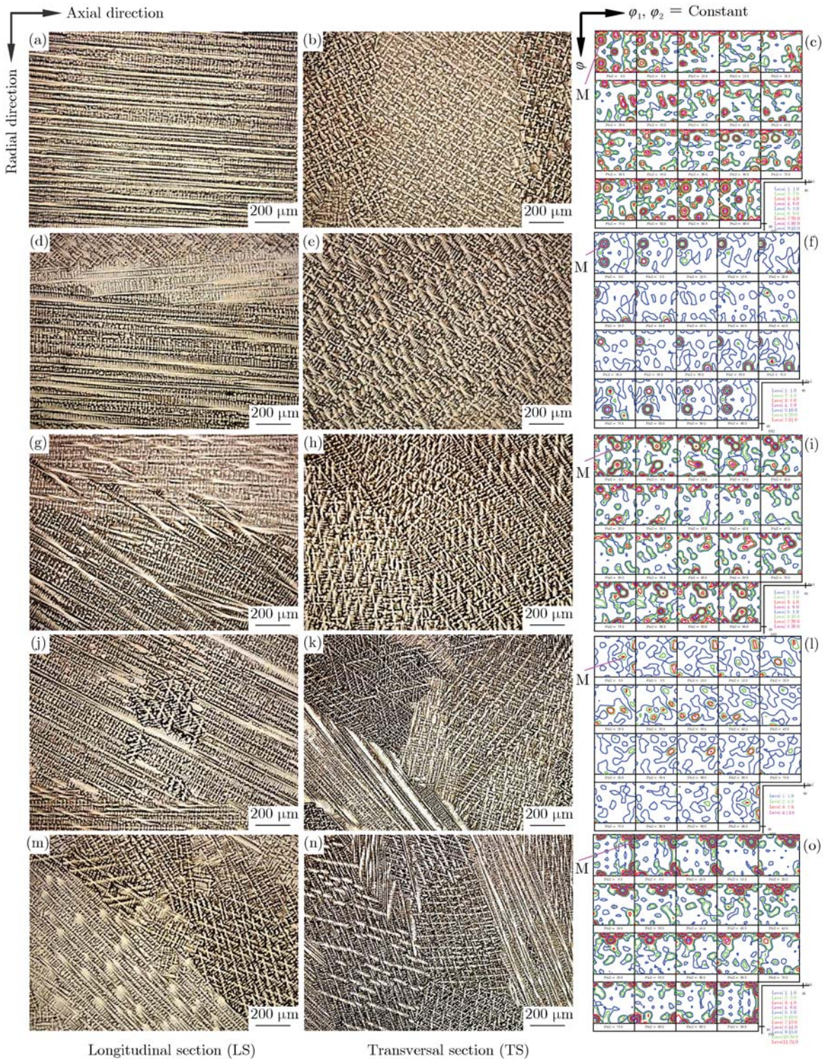
Fig. 6. Microstructures and ODFs of cast BFe10 tubes with different LSI positions in Fig. 5: (a)-(c) with position (1), (d)-(f) with position (2), (g)-(i) with position (3), (j)-(l) with position (4), and (m)-(o) with position (5). LS contains (a), (d), (g), (j), and (m); TS contains (b), (e), (h), (k), and (n). “M” in the ODF figure above represents the “main texture” as shown in Table 3.
