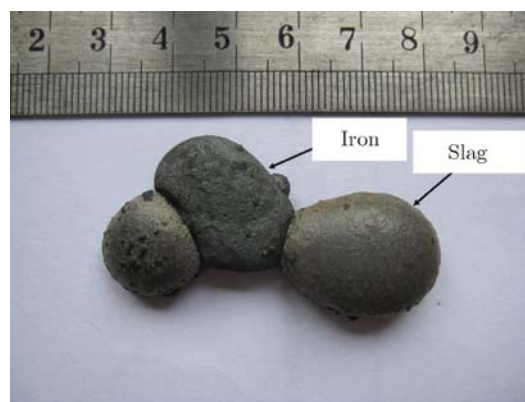
Fig. 6. Morphology of iron nugget and slag separation (anthracite, 1400°C, 15 min).
