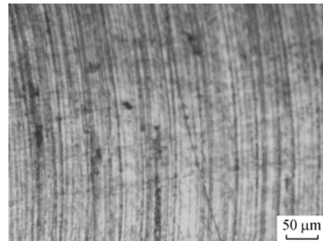
Fig. 8. Milled surface of the aluminum alloy-5wt% silicon carbide composite work piece.
