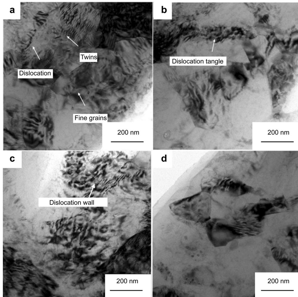
**Fig. 8** High magnification TEM images of ARB-processed Mg–5Li–1Al sheets: **a** ARB1; **b** ARB2; **c** ARB4; **d** ARB6. Reproduced with permission from Ref. [61]. Copyright 2017, Published by Elsevier Ltd on behalf of the editorial office of Journal of Materials Science & Technology
