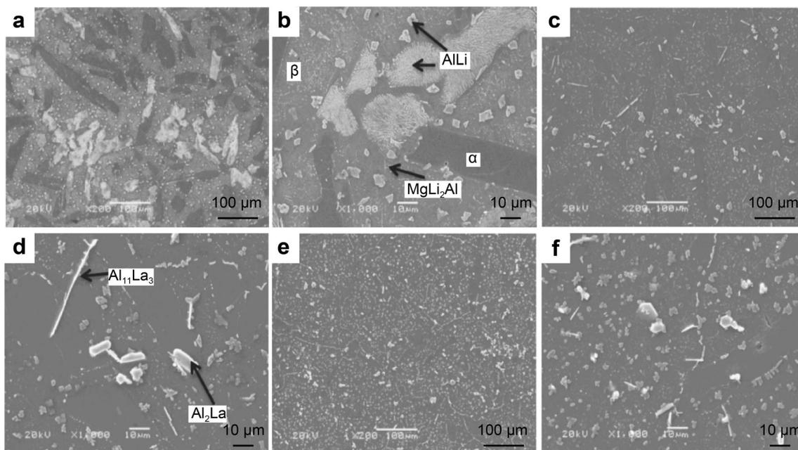
**Fig. 1** SEM images of Mg-9Li-6Al alloys with different La contents: **a, b** 0%; **c, d** 2%; **e, f** 5%. Reproduced with permission from Ref. [25]. Copyright 2014, Elsevier B.V
