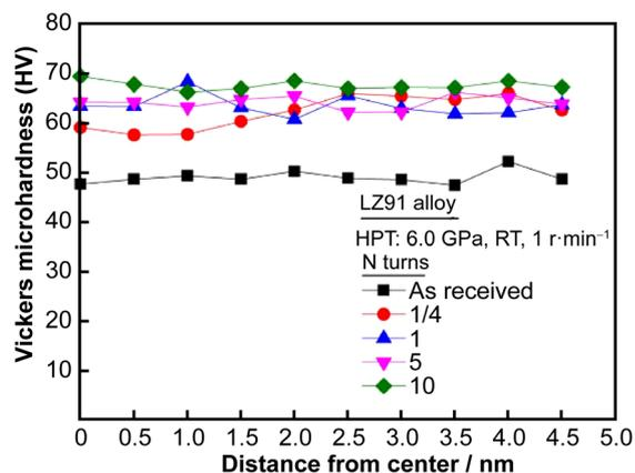
**Fig. 7** Vickers microhardness of LZ91 alloy along the radius of disk. Reproduced with permission from Ref. [60]. Copyright 2018 by the authors
