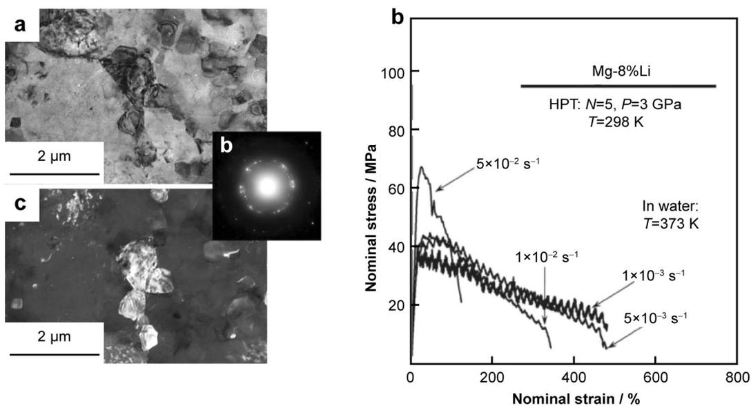
**Fig. 6** TEM observation after HPT processing 5 turns: **a** bright-field image, **b** SAED pattern, and **c** dark-field image; **d** nominal stress versus nominal strain curves obtained in boiling water for samples processed by HPT 5 turns. Reproduced with permission from Ref. [58]. Copyright, 2015 Elsevier B.V
