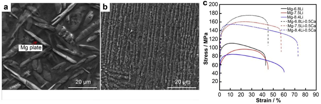
**Fig. 3** Microstructural evolution of Mg-8.4Li alloys **a** before and **b** after Ca addition; **c** corresponding room-temperature tensile engineering stress-strain curves of Mg-xLi alloys before and after Ca addition. Reproduced with permission from Ref. [36]. Copyright 2015, Elsevier B.V
