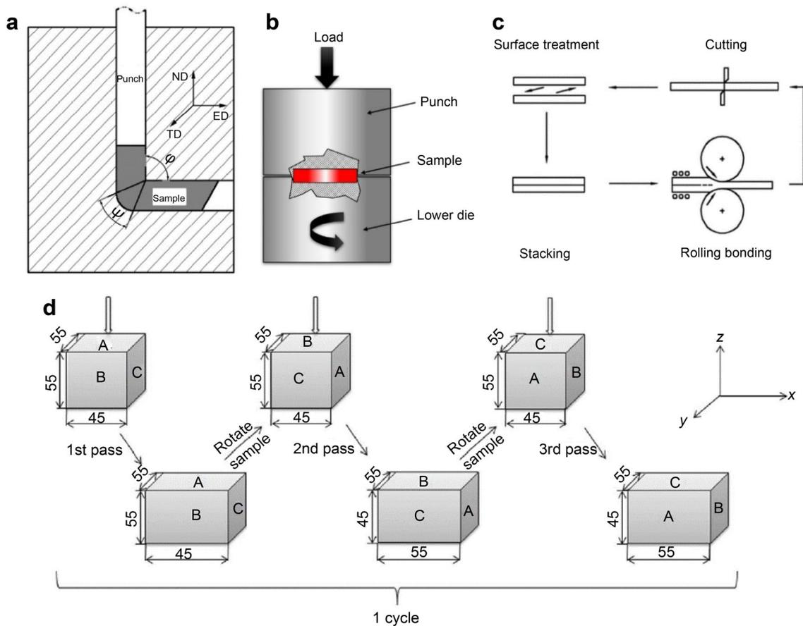
**Fig. 4** Schematic diagram of SPD techniques: **a** ECAP, **b** HPT, **c** ARB, and **d** MDF. Reproduced with permission from Refs. [50, 52–54]. Copyright 1994–2021, China Academic Journal Electronic Publishing House; Copyright 2015, WILEY-VCH Verlag GmbH & Co. KGaA, Weinheim; Copyright 2018, WILEY-VCH Verlag GmbH & Co. KGaA, Weinheim; Copyright 2016, the Indian Institute of Metals - IIM
