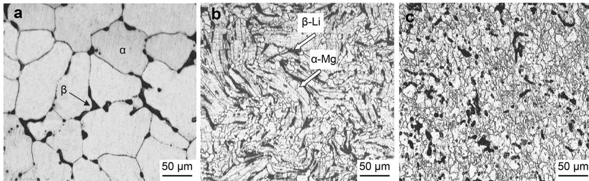
**Fig. 5** Micrographs of LZ61 alloy for **a** as-cast, **b** extruded and **c** ECAPed conditions. Reproduced with permission from Ref. [55]. Copyright 2013, The Minerals, Metals & Materials Society and ASM International
