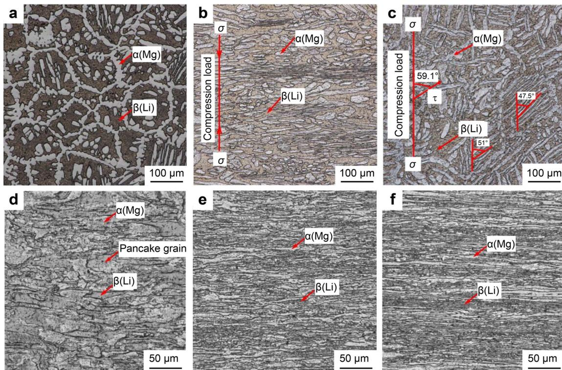
**Fig. 9** OM images of Mg–10.2Li–2.1Al–2.23Zn–0.2Sr alloy at different status: **a** as-cast; **b** 1st pass of MDF, 573 K, pass strain of 0.5; **c** 6th pass of MDF, 573 K, accumulative strain of 3.0; **d** cold rolling, ND; **e** cold rolling, TD; **f** cold rolling, RD. Reproduced with permission from Ref. [48]. Copyright 2017, Elsevier B.V
