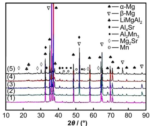
**Fig. 2** XRD patterns of different alloys: (1) Mg-8Li-3Al-0.5Mn; (2) Mg-8Li-3Al-0.5Mn-0.25Sr; (3) Mg-8Li-3Al-0.5Mn-0.5Sr; (4) Mg-8Li-3Al-0.5Mn-0.75Sr; (5) Mg-8Li-3Al-0.5Mn-1.0Sr. Reproduced with permission from Ref. [26]. Copyright 2014, the Nonferrous Metals Society of China
