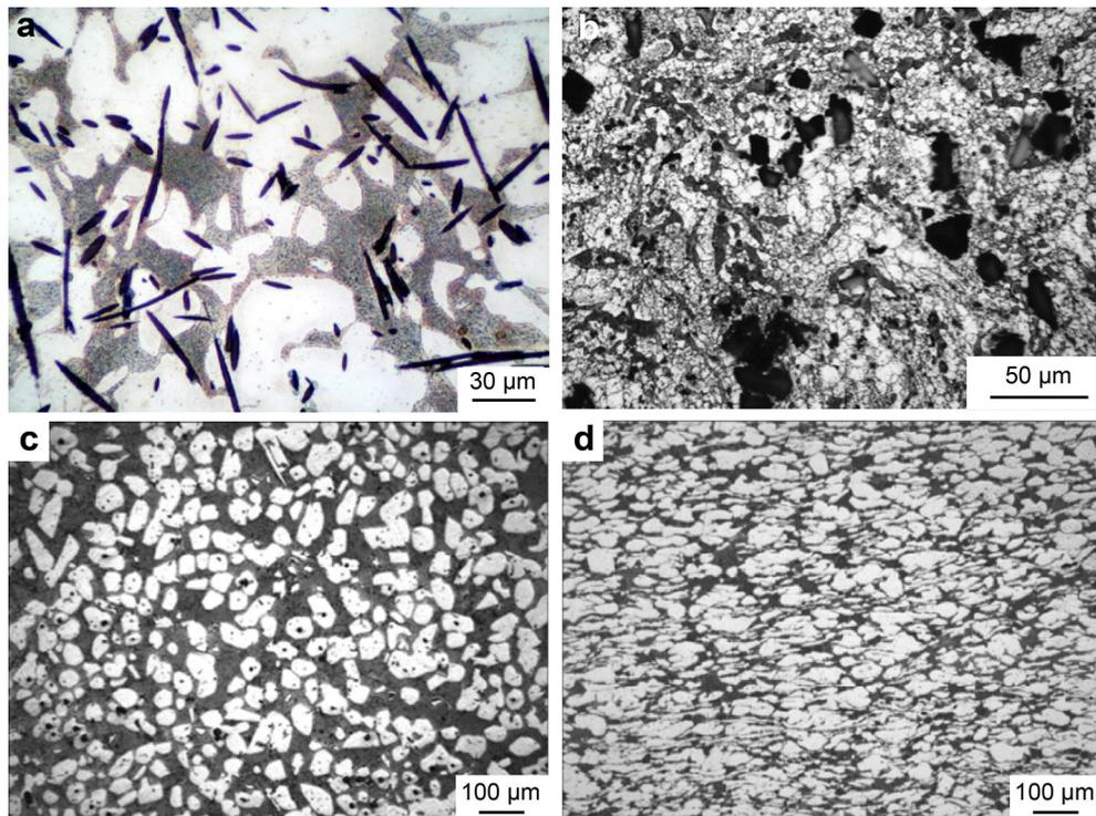
**Fig. 10** Microstructures of Mg–8Li with **a**  $\delta$ -Al<sub>2</sub>O<sub>3</sub> fiber, **b** SiC particles, **c** as-cast Mg–8Li–1Al–1Y alloy and **d** B<sub>4</sub>C<sub>p</sub>/Mg–8Li–1Al–1Y composite. Reproduced with permission from Refs. [19, 65]. Copyright 2006, Elsevier Ltd.; Copyright 2011, the Nonferrous Metals Society of China
