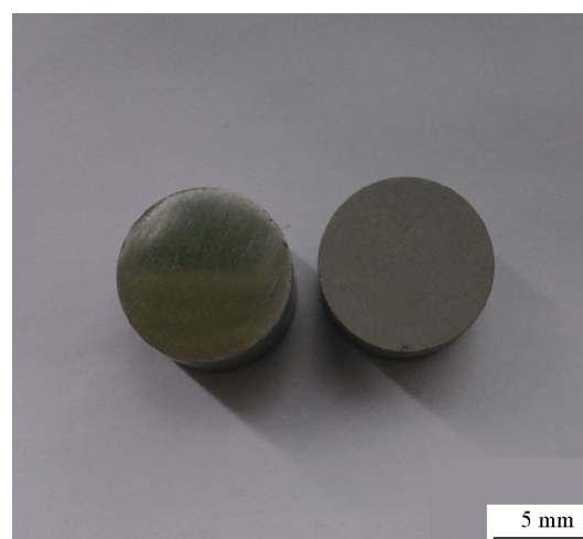
Fig. 5 Macro-photographs of phosphated and no phosphated samples at 2 min in salt spray test
