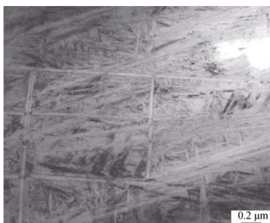
Fig. 3 TEM image of \alpha' martensite in TACF alloy solution treatment at 1233 K for 30 min after WQ
