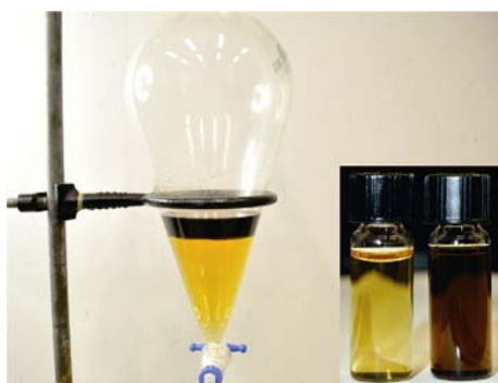
Fig. 2 Photograph showing the extraction result of Pt NPs from the dissolved Au after the leaching process: the bottom phase being the acetonitrile solution with dissolved Au; the upper phase is the extracted Pt NPs dispersed in hexane. (The two layers can be easily separated (inset))
