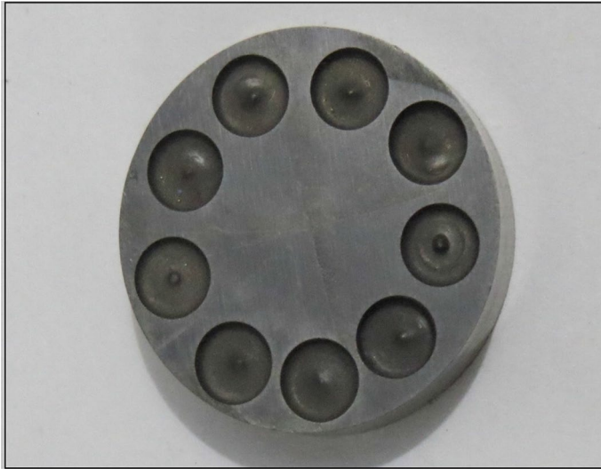
Fig. 3 Holes drilled in workpiece during pilot experiments
