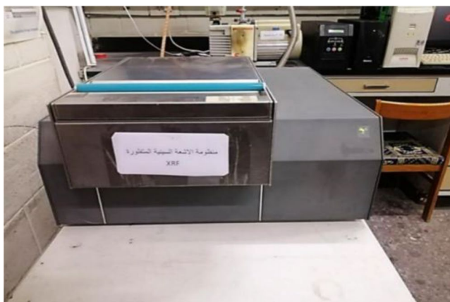
Fig. 3 XRF system used for experiment
