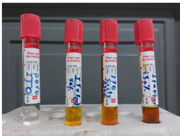
Fig. 1 Shows from left; pure ITO solution and ITO with different mixing ratios of \text{FeCl}_3 , 50, 100, and 150% respectively
