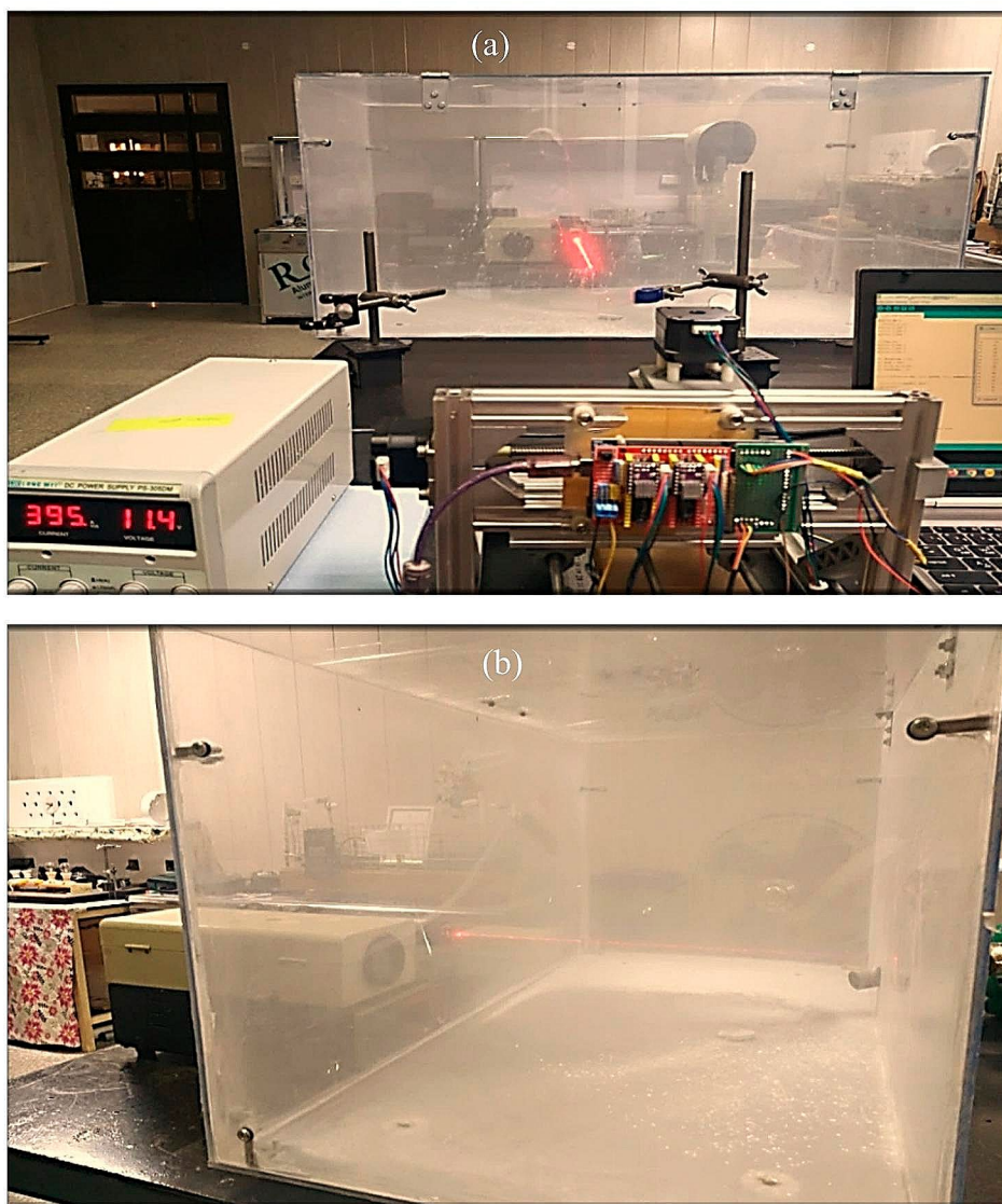
Fig. 4 Laser beam transmissions over dust (a) front view (b) side view
