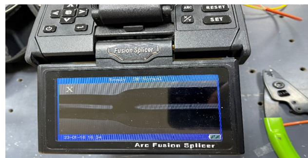
Fig. 2 Splicing of PCF and SMF by means of fusion splicer
