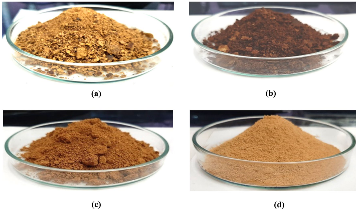
Fig. 1 Pomegranate peel powder subjected to different drying techniques. Hot air oven dried a , Microwave dried b , sun dried c , freeze dried d
