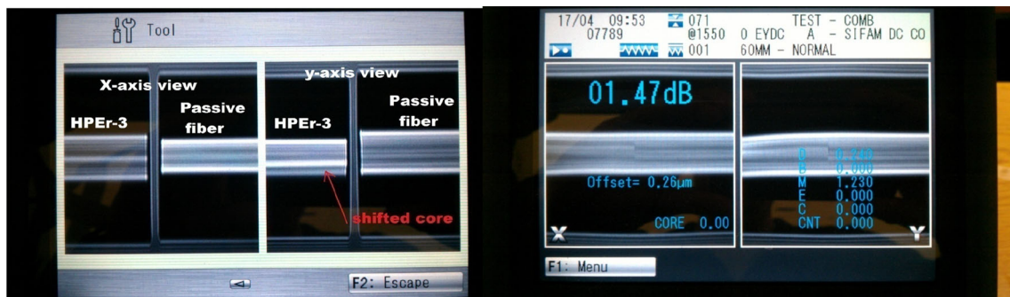
Fig. 10 Picture showing the core mismatch between passive and Hexagonal shaped low RI coated fiber with the splicing loss 01.47 dB
