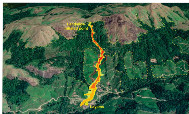
Fig.2. Pre-event Google Earth image showing the location of landslides. Landslide runout was modeled using Laharz and draped over Google Earth image. Yellow dotted line indicates boundary between different land use category and red line indicates the suspected landslide.
