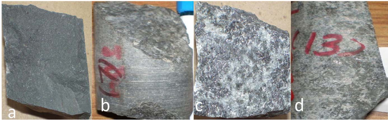
Fig.4. (a) Olivine (micro) dolerite KHR- 10/216.40. (b) Hypersthene dolerite KHR-4/227.15. (c) Olivine norite KHR-10/300.00. (d) Norite KHR-5/299.00.
