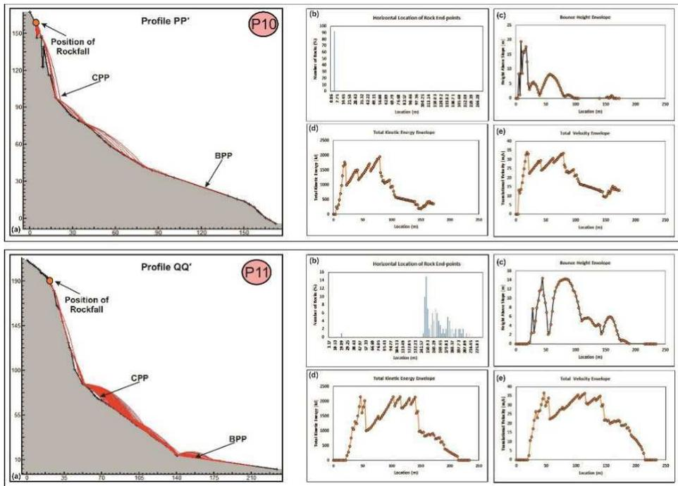
**Fig.6.** Rockfall analysis for profile PP' and QQ': (a) trajectory path; graph of (b) runout versus distance; (c) bounce height versus distance; (d) maximum kinetic energy versus distance; (e) translation velocity versus distance.
