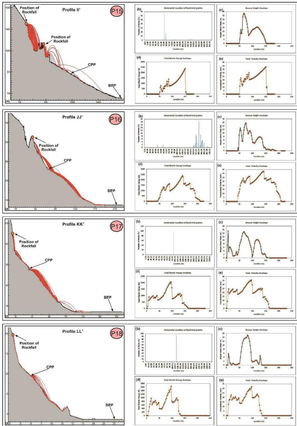
**Fig.8.** Rockfall analysis for profile II' to LL': (a) trajectory path; graph of (b) runout versus distance; (c) bounce height versus distance; (d) maximum kinetic energy versus distance; (e) translation velocity versus distance.
