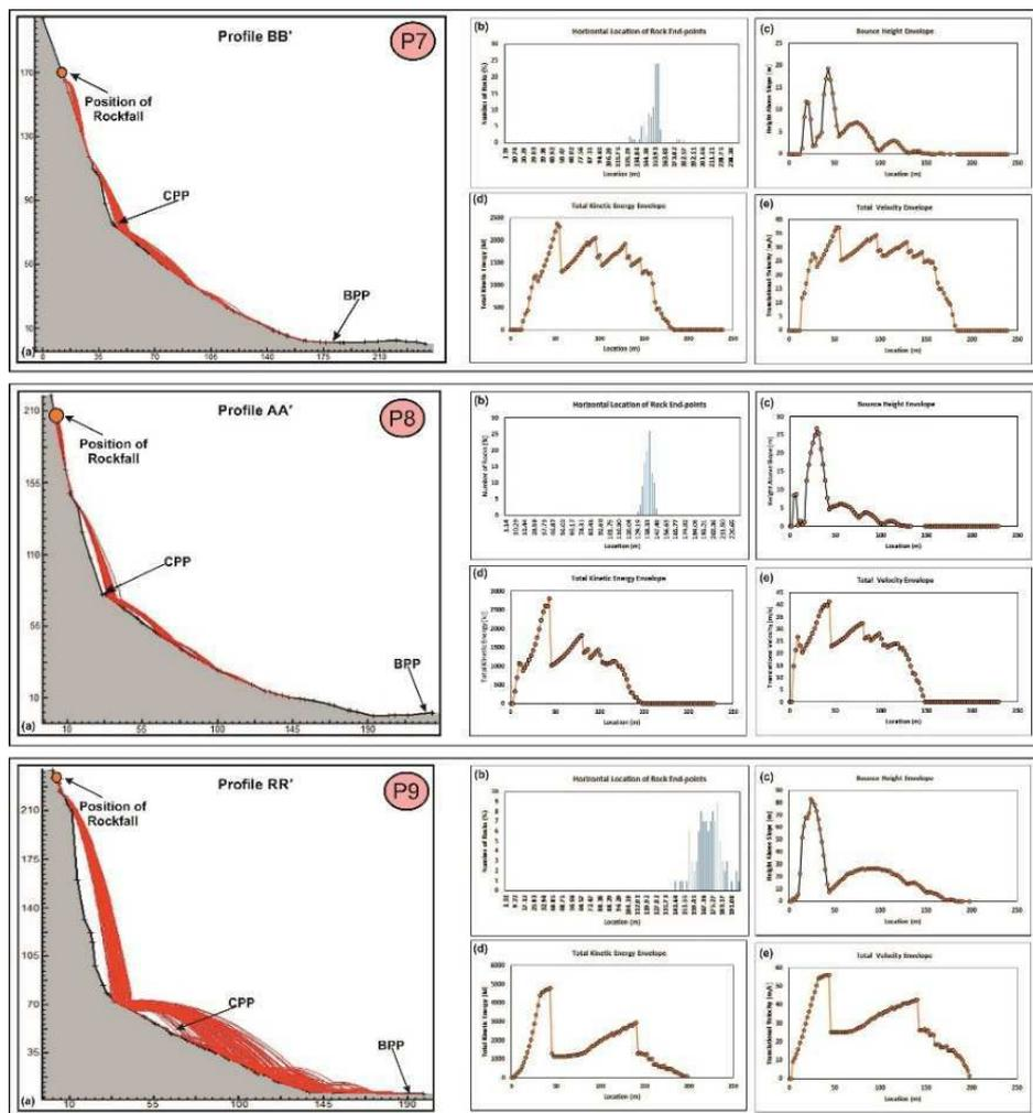
**Fig.5.** Rockfall analysis for profile BB', AA' and RR': (a) trajectory path; graph of (b) runout versus distance; (c) bounce height versus distance; (d) maximum kinetic energy versus distance; (e) translation velocity versus distance.
