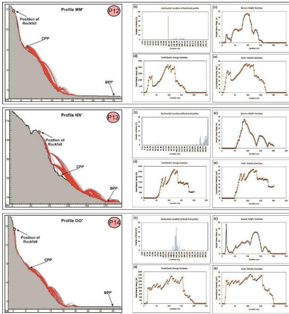
**Fig.7.** Rockfall analysis for profile MM', NN' and OO': (a) trajectory path; graph of (b) runout versus distance; (c) bounce height versus distance; (d) maximum kinetic energy versus distance; (e) translation velocity versus distance.
