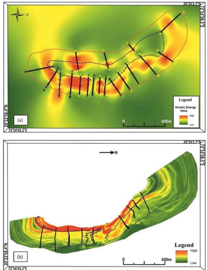
**Fig.9.** Energy Map showing concentration near the parikrama path (a) derived from 2D Rocfall program (b) derived from 3D Rockfall Analyst program.
