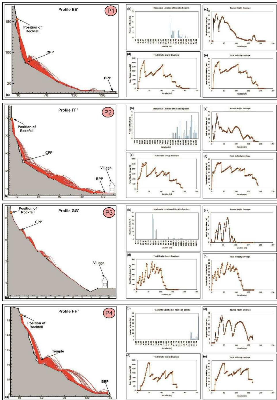
**Fig.3.** Rockfall analysis for profile EE' to HH': (a) trajectory path; graph of (b) runout versus distance; (c) bounce height versus distance; (d) maximum kinetic energy versus distance; (e) translation velocity versus distance.
