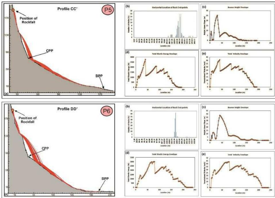
**Fig.4.** Rockfall analysis for profile CC' and DD': (a) trajectory path; graph of (b) runout versus distance; (c) bounce height versus distance; (d) maximum kinetic energy versus distance; (e) translation velocity versus distance.
