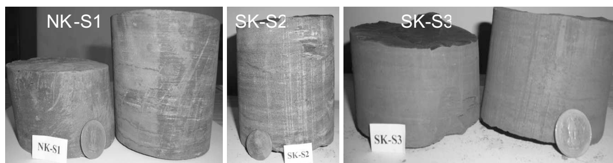
Fig.2. Megascopic photographs of shale core samples obtained from North and South Karanpura coalfields (Sample NK –S1, SK-S2 and SK-S3).
