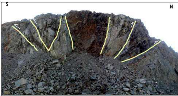
Fig.3. Flower faults structure in southwest wall of the Gole Gohar mine.
