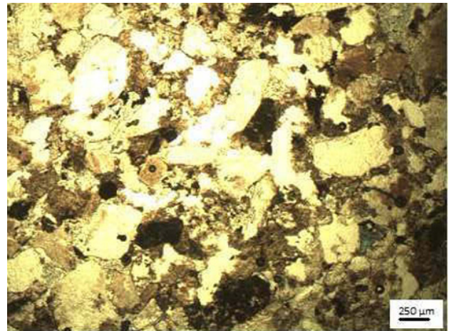
Fig.12. Microphotograph shows laminated fine to medium-grained sandstone/siltstone facies (F4). Quartz grains are ill-sorted, sub-angular to sub-rounded and aligned parallel to the lamination, (a) at R1 S-2 location), (b) at R3 S-6. location.
