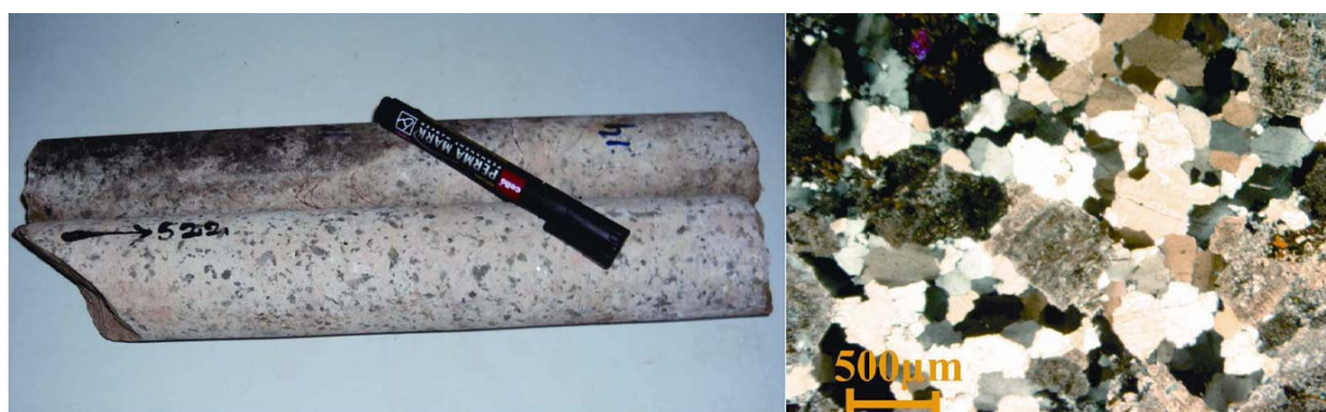
Fig.2. Examples of collected granite cores and a generalized photomicrograph of the granite.
