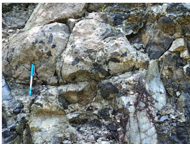
Fig.2. Field photograph of mineralised breccia zone containing clasts of ferritchromit in medium grained gabbro matrix. (Bangur quarry)
