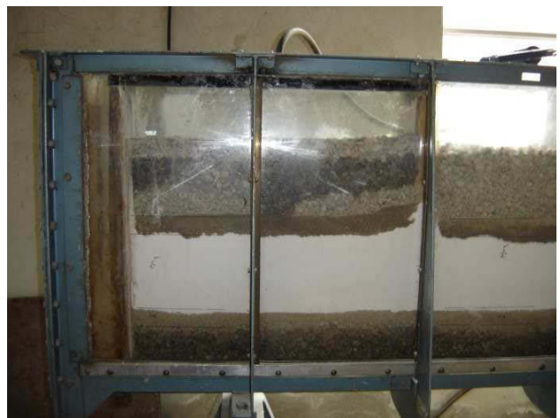
Fig.2. Soil classification in model of dam foundation (a) schematic. (b) actual (Dimensions are in term of centimeter)
