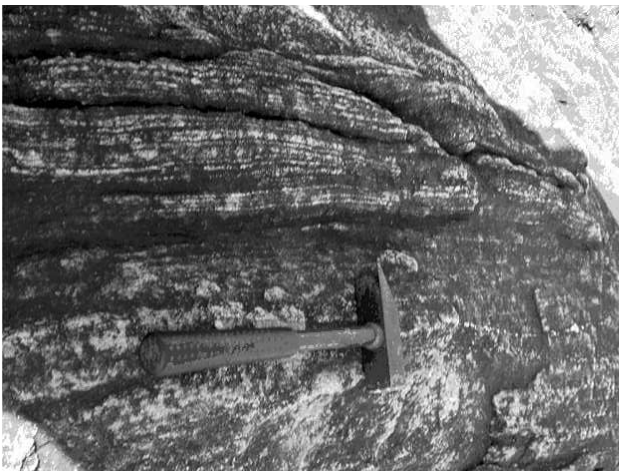
Fig.9. Weathered foliation in granite gneiss – possible seepage pathway of groundwater.
