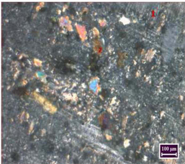
Fig.8. Granite-gneiss under cross polarized light. Plagioclase (1) and biotite (2) are demarcated in granite.
