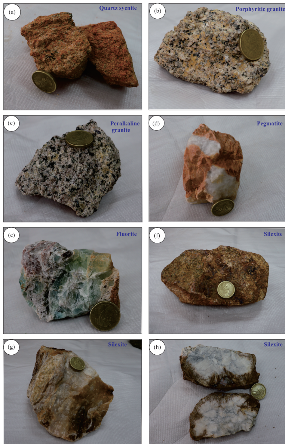
Figure 3. Hand specimen photographs of the studied rocks: (a) quartz syenite, (b) porphyritic granite, (c) peralkaline granite, (d) pegmatite, (e) fluorite, (f) dark-brown silixite, (g) yellowish-brown silixite, and (h) whitish-gray zoned silixite.
