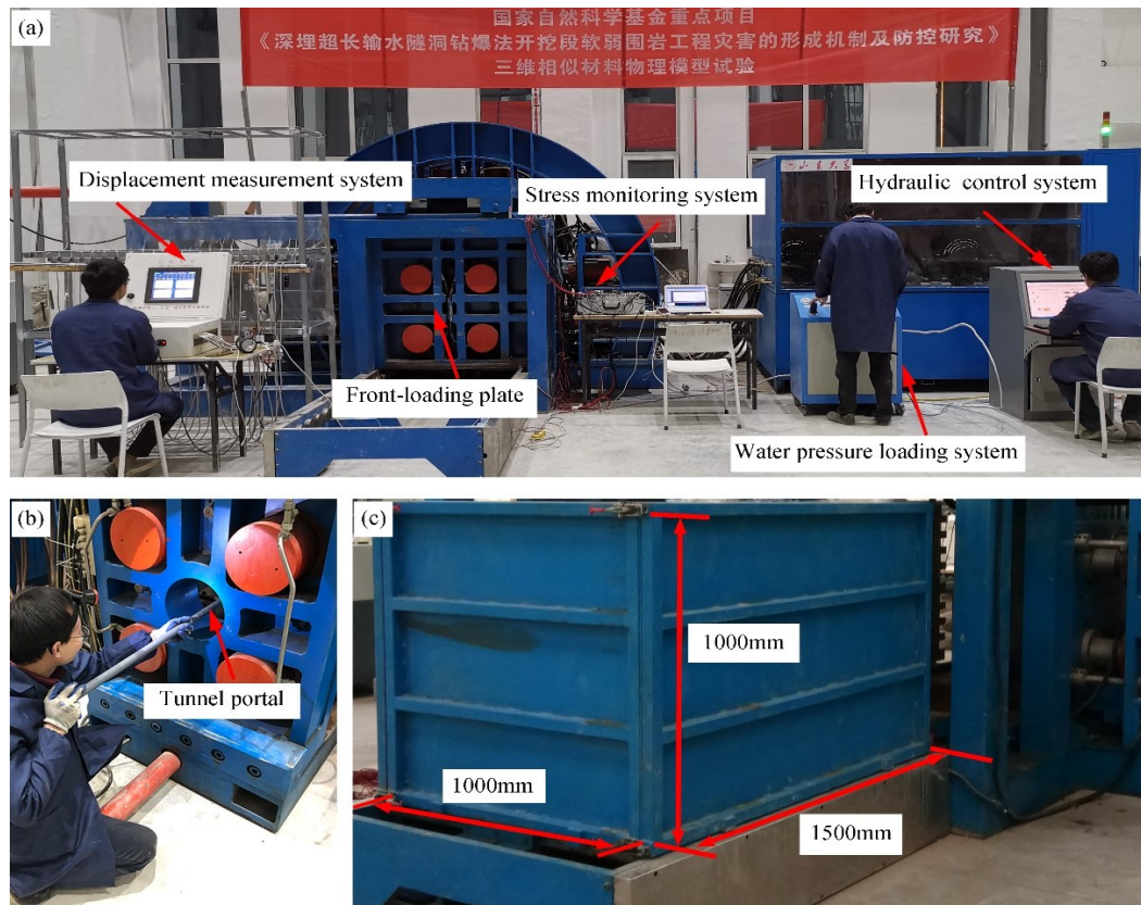
Figure 4. The true triaxial physical model test system. (a) The model test apparatus; (b) back-loading plate; (c) the box mold.
