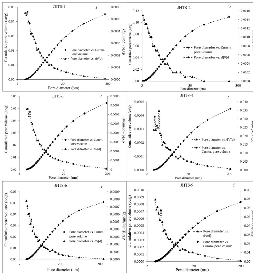
**Figure 13.** Estimation of pore size distribution in shale core samples by BJH method.
