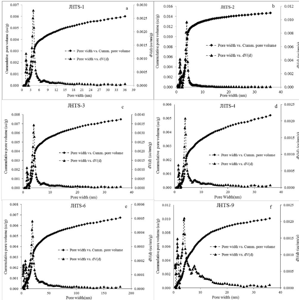
Figure 14. DFT plots for determination of surface area, pore size and pore volume of shale core samples.
