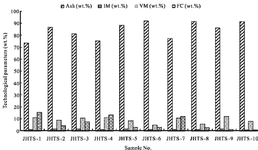
Figure 2. Distribution of technological parameters in shale cores samples.
