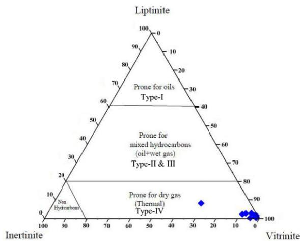
**Figure 6.** Ternary diagram of maceral distribution illustrating Barakar shale of Jharia are placed in thermal-dry gas prone region.
