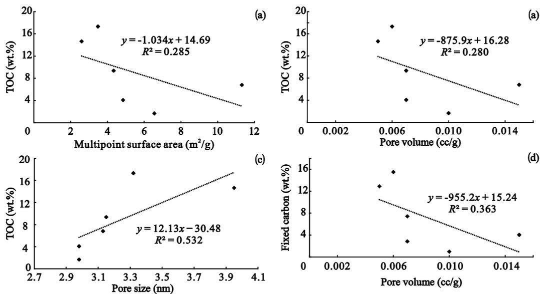
Figure 17. Plot of (a) multipoint BET surface area vs. TOC, (b) pore volume vs. TOC, (c) pore size vs. TOC, (d) pore volume vs. fixed carbon.
