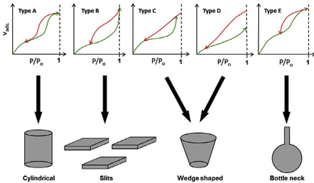
Figure 10. Different types of hysteresis pattern representing their pore geometrical shapes (after Labani et al., 2013; de Boer, 1958).
