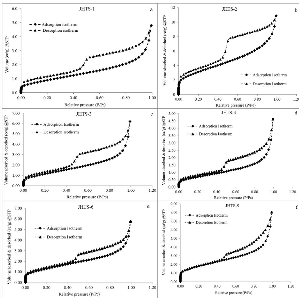
Figure 11. Low pressure  $N_2$  sorption isotherm of Barakar shale core samples (a) cylindrical-type A; (b) large spaced open slit pores-type B; (c) cylindrical-type A; (d), (e) and (f) bottle-neck-type E.
