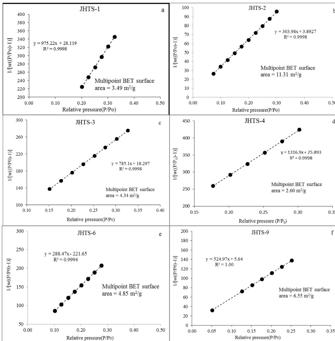
Figure 12. Multipoint BET plots for surface area determination of shale core samples.
