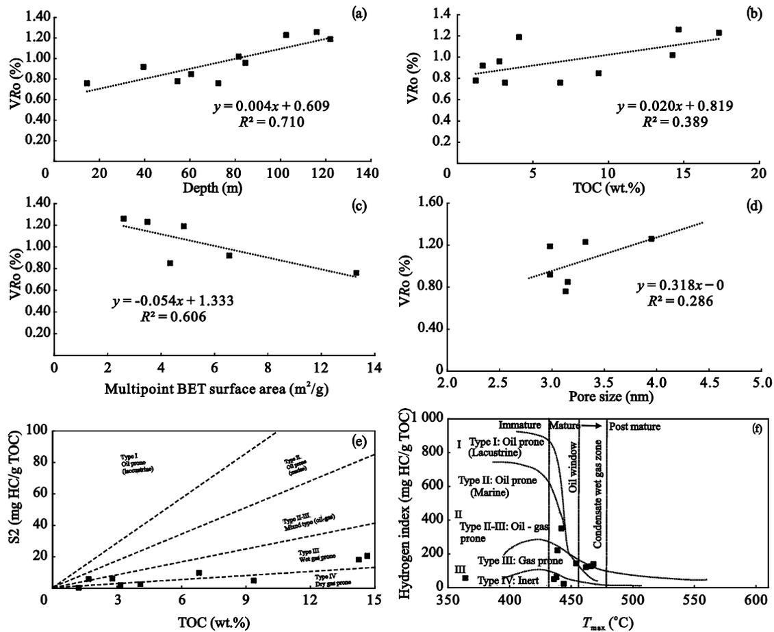
Figure 16. Plot of (a) depth vs. VRo, (b) TOC vs. VRo, (c) multipoint BET surface area vs. VRo, (d) pore size vs. VRo, (e) TOC vs. S2 and (f)  $T_{max}$  vs. HI.
