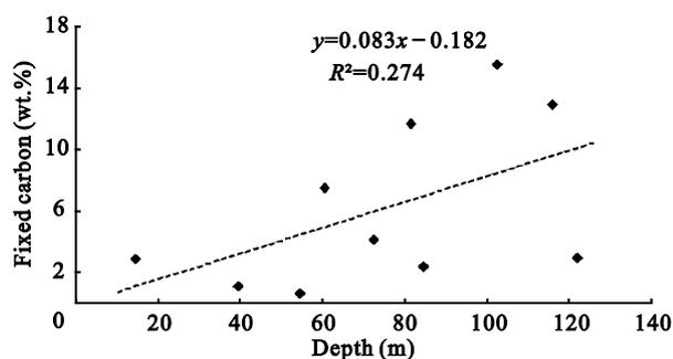
Figure 3. Increasing trend of fixed carbon with depth.
