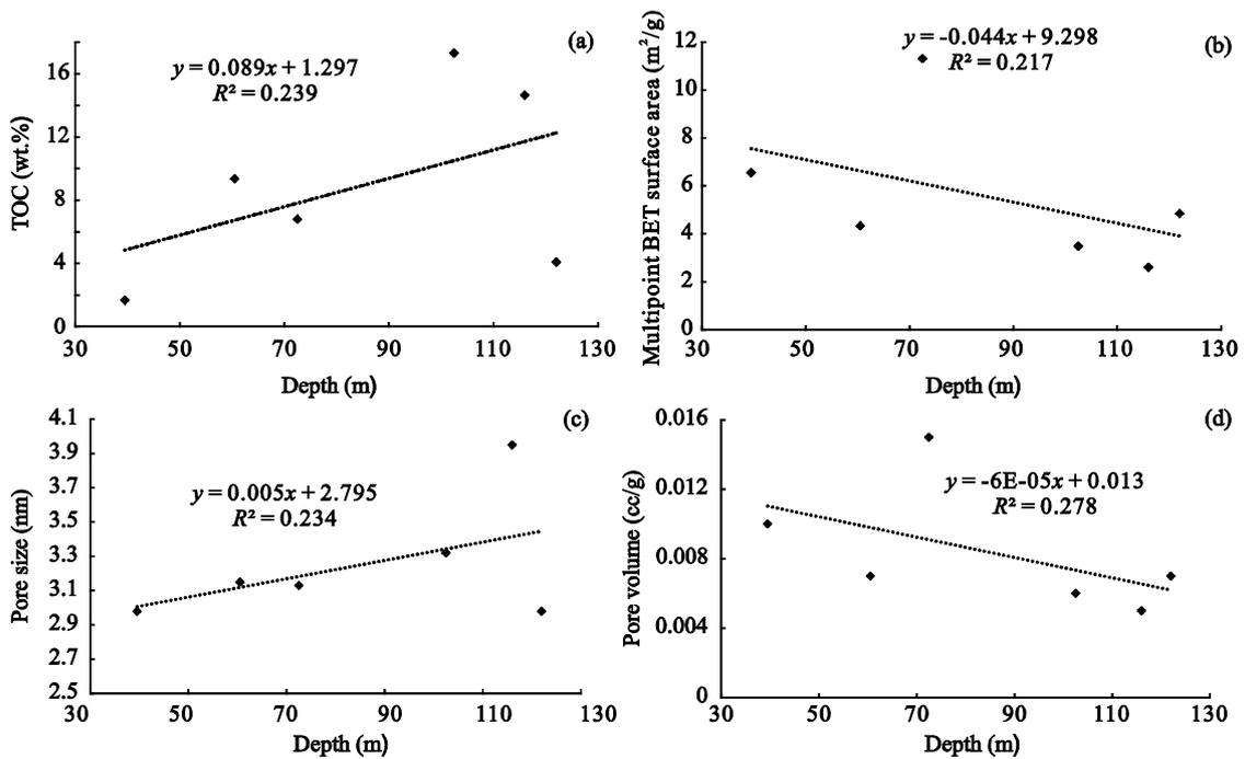
Figure 15. Plot of (a) depth vs. TOC, (b) depth vs. multipoint BET surface area, (c) depth vs. pore size, (d) depth vs. pore volume.
