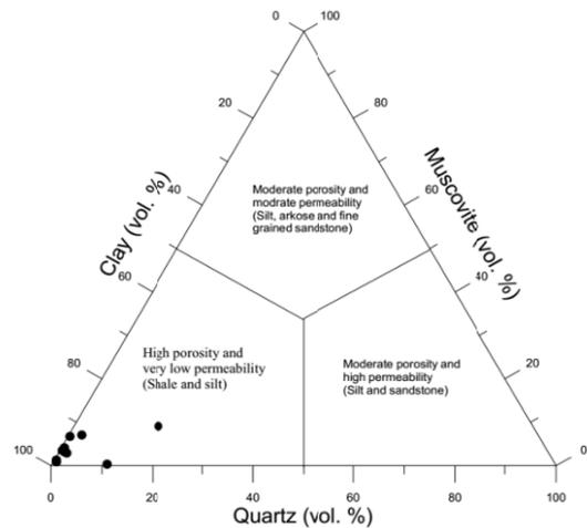
**Figure 7.** Ternary diagram of mineral distribution showing likely porosity and permeability based on weathering pattern of deposition.
