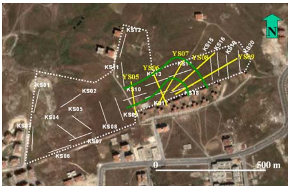
Figure 2. Location map for the seismic survey conducted within the residential development project site. The survey consisted of refraction profiling at 20 locations (KS01–20) and reflection profiling along five line traverses (YS05–09). The white lines denote the orientation of the receiver spreads for the refraction survey. The green curves denote the extremities of the landslide failure zone.
