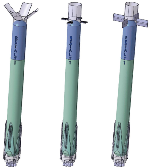
Fig. 1 First stage of RETALT1 configuration with different aerodynamic control surfaces (from left to right): petals, grid fins, planar fins
