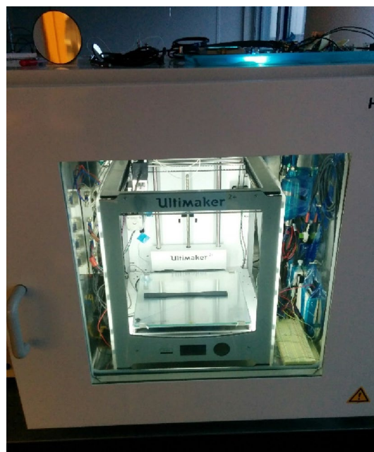
Fig. 1 Experimental set up showing the 3D printing inside the vacuum chamber and the electrical connection routing needed to reconnect the printer to the electronic and power board located outside the chamber
