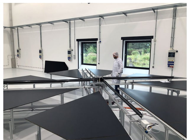
Fig. 8 Boom Spool Deployer Ambient Deployment ( © HPS GmbH)
