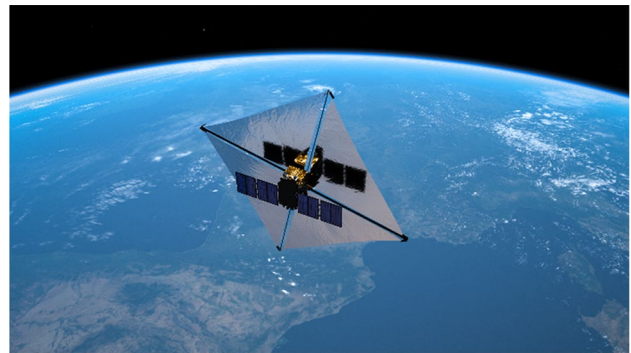
Fig. 3 Animated view of deployed ADEO-L, ©Platform P200 (QinetiQ Space), ©De-Orbit System (HPS GmbH)
