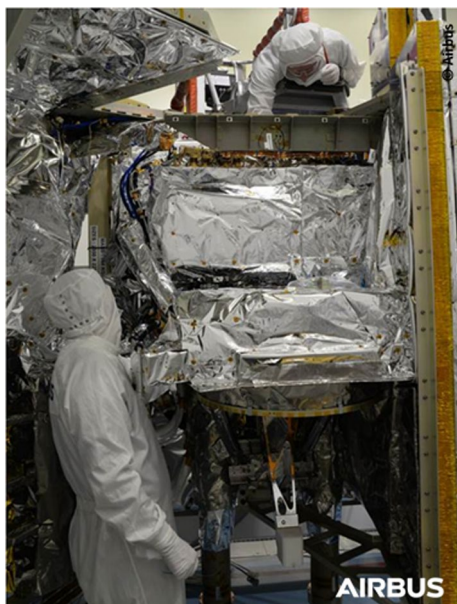
Fig. 14 Integration of LCS evaporators on PLH's back wall, with ATLID pointing downwards
