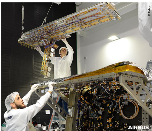
Fig. 12 LCS integration on ATLID HSA
