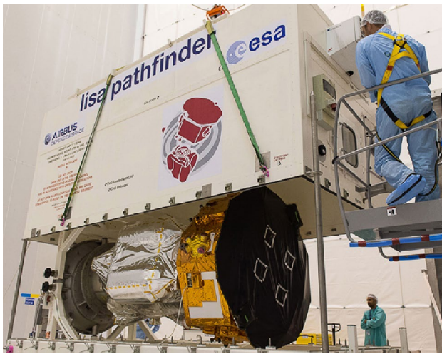
Fig. 1 Unpacking of the LISA Pathfinder spacecraft after arrival at Europe's spaceport in Kourou, French Guiana. The propulsion module (left) and the science module (right) are shown
