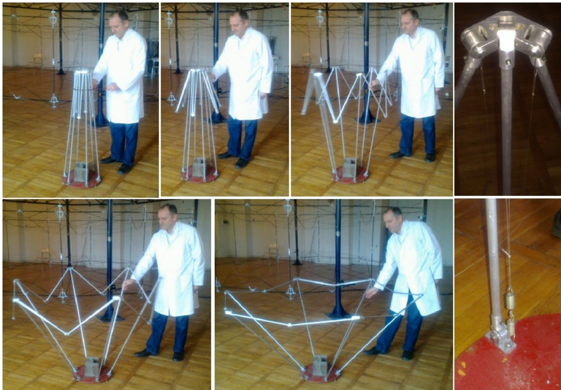
Fig. 6 The single-ring cone structure with brackets and V-folding rods turned inside out where the struts are connected to the upper corner brackets using cylindrical hinges with rotation axis tangential to the ring
