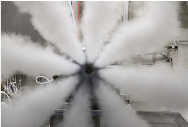
Fig. 14 Test with \text{H}_2\text{O}_2 catalyst chamber carried out in March 2013 (mass flow 120 g/s)
