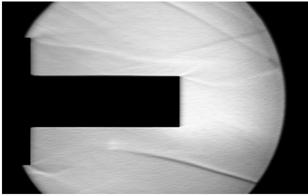
Fig. 19 Averaged Schlieren image without jet flow ( p_{t,\infty} = 1.5 bar, T_\infty = 285 K and M_\infty = 2.9 )
