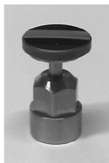
Fig. 5 Picture of the test tool showing the Si-IR lens on top glued to the adapter for the UNAT tester and 3D plot of the interferometric determination of the surface topology of the used Si-IR lens
