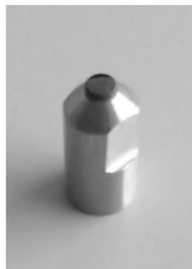
Fig. 6 Picture of the test tool showing the polished manufactured SiC lens on top of the test tool and 3D plot of the interferometric determination of the surface topology of the used SiC lens
