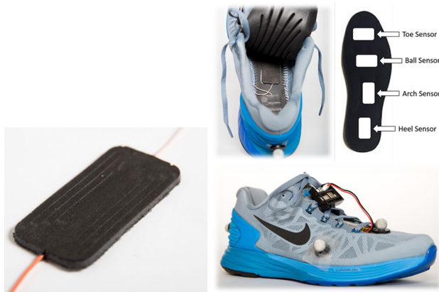
Fig. 2 In-shoe sensor: (Left) NCPF sensor with wires embedded to measure the voltage response during impacts. (Right) Shoe equipped with NCPF foam sensors, microcontroller, and battery. The sensors were embedded under the insole at the heel, arch, ball, and toe
