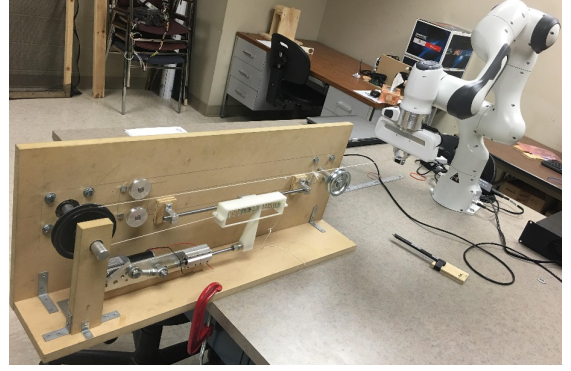
Fig. 6. Experimental setup with the fabricated prototype of the series-elastic mechanism for back-pain rehabilitation and a robotic manipulator.
