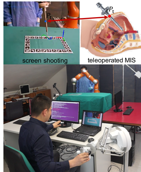
Fig. 7. Operative step using the Kuka LWR 4+ robot.
