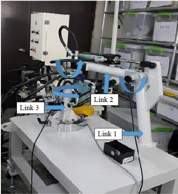
Fig. 16. Structure of three link hydraulic servo system.
