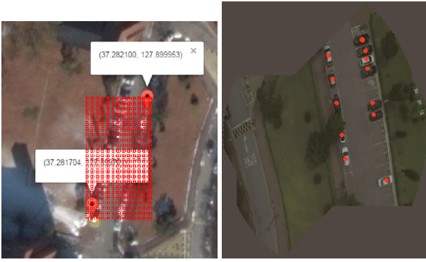
(a) Google map showing the start and end locations including the targets manually selected and their latitudes and longitudes. (b) Image mosaic including the targets and represented by the red dots.
