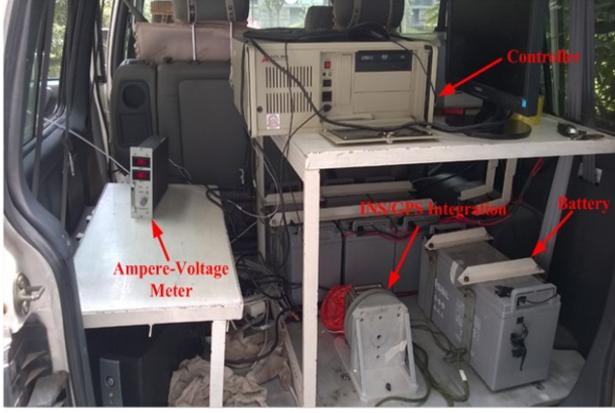
Fig. 5. Experimental setup for the vehicle navigation.
