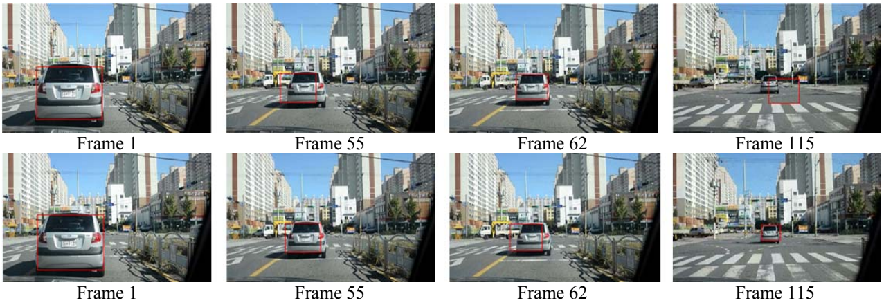
Fig. 13. Tracking comparison results: with(bottom) and without(top) color histogram updating.
