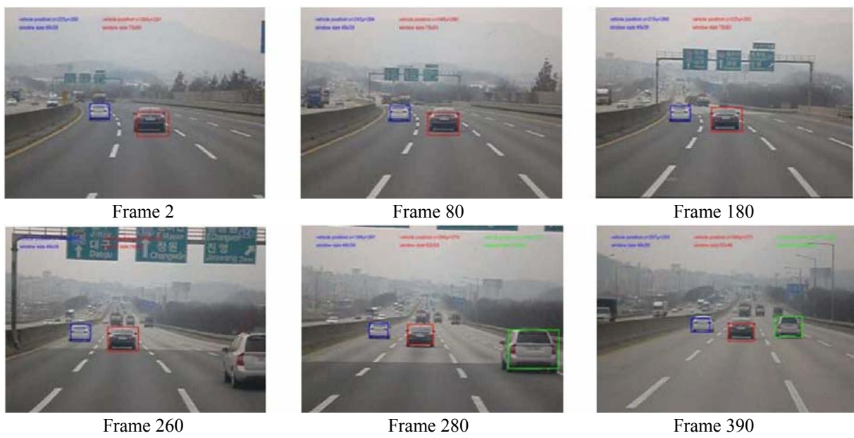
Fig. 15. Multiple vehicle detection and tracking.
