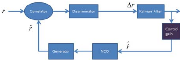
Fig. 3. The signal tracking loop using the LQG regulation gain.
