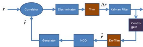
Fig. 4. The moving set-point signal tracking loop using LQG.
