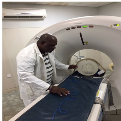
Fig. 2 Set up for measuring CTDI
