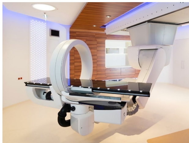
Fig. 10 Irradiation room and patient positioning system. The imaging ring mounted on the couch is used for the precise in room evaluation of the patient positioning
